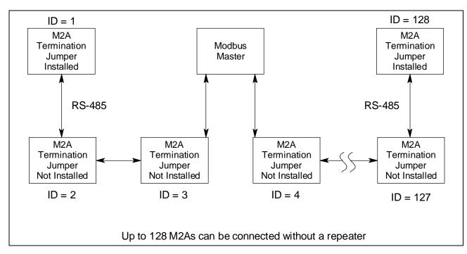
Figure 35: Multiple M2As in a Two Branch Configuration
