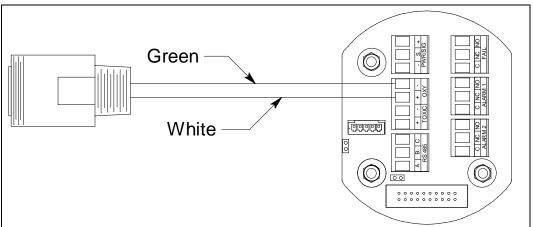
Figure 23: Partial Pressure Oxygen Detector Wiring
