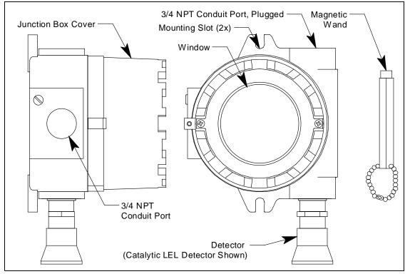
Figure 1: M2A External Components
