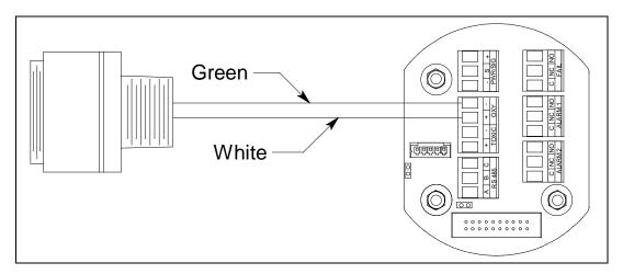
Figure 25: Capillary Type Replaceable Sensor Oxygen Detector Wiring
