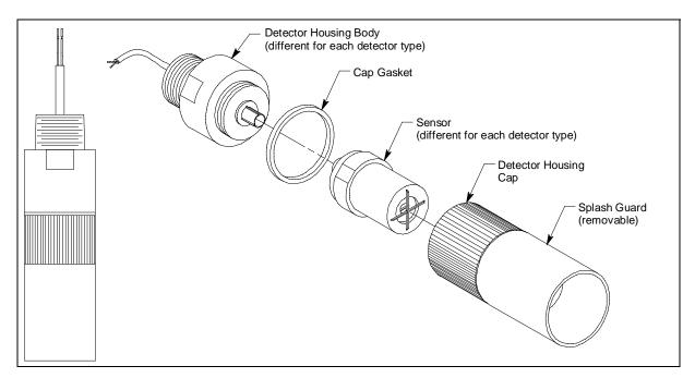
Figure 7: ESM-01 Type Detector
