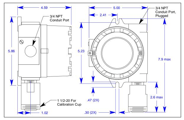
Figure 16: Outline & Mounting Dimensions, Oxygen, Partial Pressure Type
