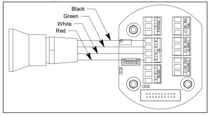
Figure 21: Catalytic LEL and ppm Detector Wiring
