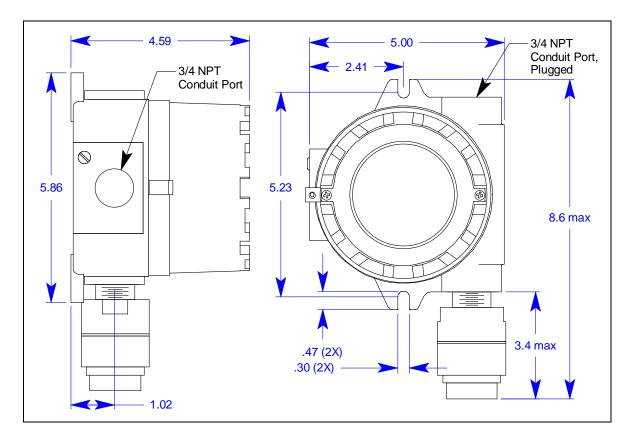
Figure 18: Outline & Mounting Dimensions, H<sub>2</sub>S, CO, and Oxygen, CSA, Explosion-Proof
