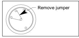
Figure 31: Plug-In Sensor Jumper Removal
