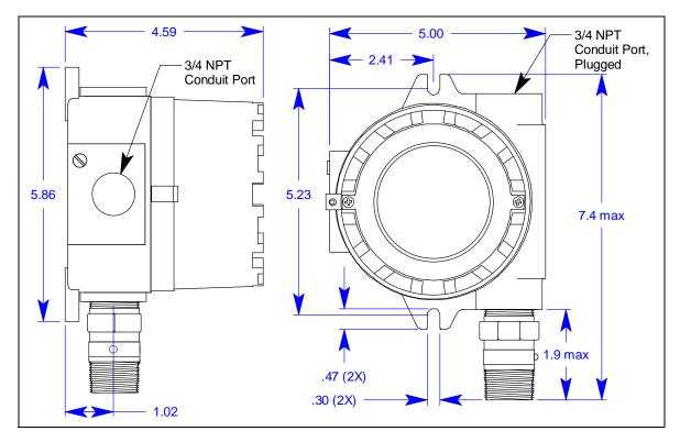
Figure 15: Outline & Mounting Dimensions, IR Combustible & CO<sub>2</sub>
