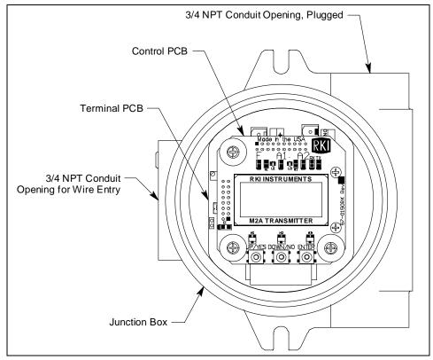
Figure 9: M2A Internal Components
