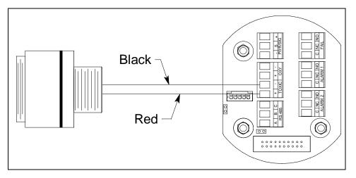
Figure 27: H<sub>2</sub>S/CO Detector Wiring
