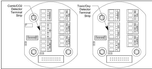
Figure 11: Detector Terminal Strip
