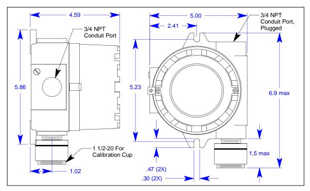
Figure 17: Outline & Mounting Dimensions, Replaceable Sensor, H<sub>2</sub>S, CO, and Oxygen, Non Explosion Proof
