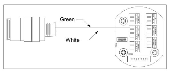
Figure 24: CSA Capillary Type Oxygen Detector Wiring
