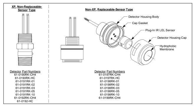
Figure 3: Infrared (IR) Sensors
