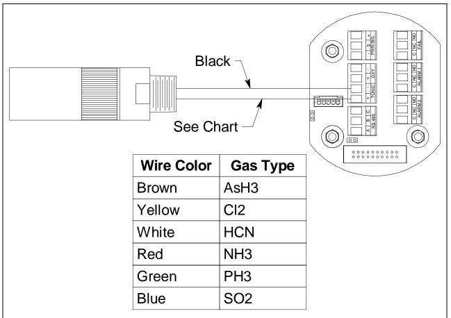
Figure 28: ESM-01 Toxic Detector Wiring
