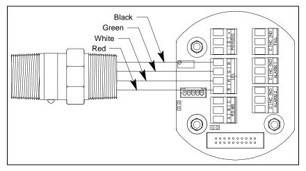
Figure 22: IR Combustible/IR CO<sub>2</sub> Detector Wiring
