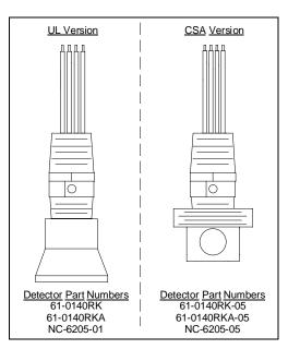
Figure 2: Catalytic Sensors
