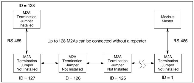
Figure 34: Multiple M2As in a Daisy Chain Configuration
