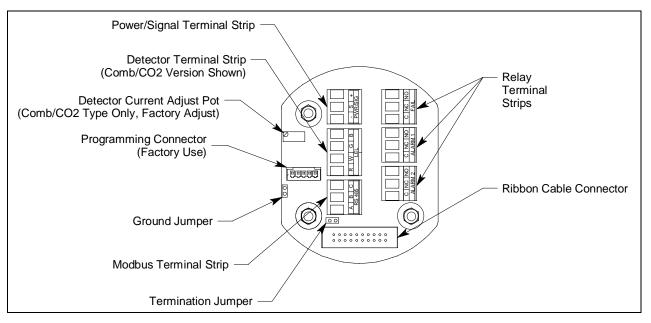
Figure 10: Terminal PCB Component Location
