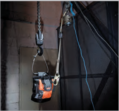
DYNAMIC TESTING Containers should have drop testing done as well including attachment points meant to anchor lanyards.
