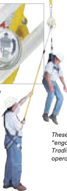
Fall arrest mode Assisted rescue by pole
