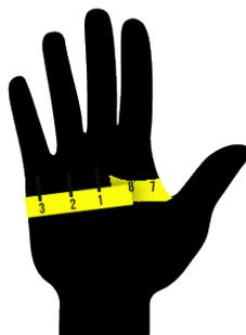
In order to determine the proper size for Class 0 and 00 insulating gloves, use a tape measure to find the circumference of your hand around the palm.
