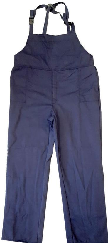
Our 8-43 cal arc flash bib overalls are made from varying weights and layers of UltraSoft® fabric, a fire-resistant blend of 88% cotton and 12% nylon. They feature leg slits and a side closure at waist, both with Velcro® closures. The straps on the overalls have a criss-cross back with plastic crosser, and plastic Nexus® clip closure at upper chest.
