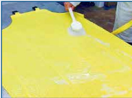
A liquid dishwashing detergent is most effective as a degreasing and cleaning agent.
