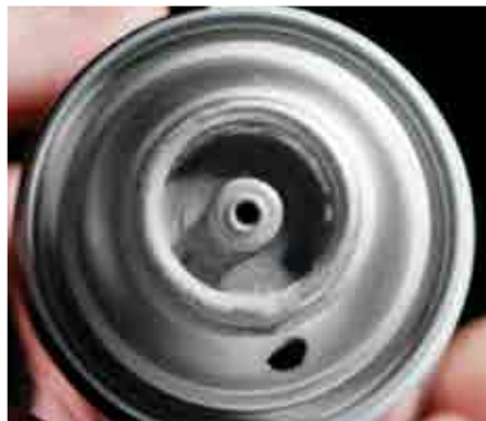
Smooth side puncture leaves no jagged edges.
